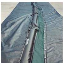
Floating Turbidity Control Curtains are impermeable barriers\* constructed of a flexible reinforced thermoplastic material dielectrically welded to provide an upper hem for enclosing flotation material and a lower hem for enclosing ballast material. The skirt depth of the silt curtain is the material vertically below the upper hem. The length of the turbidity curtain is the horizontal distance between ends. Additional construction features are dependent on silt curtain design.
